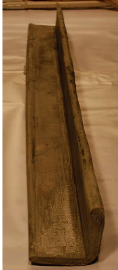
Cross section of pultruded shapes with TRC laminates
